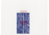
0.005" (0.127mm) wide 110# REFLECTION @ 2200 fpm (670 m/min) One Coating Scratch Detected by the OPTOMIZER
