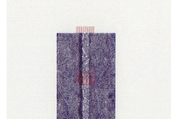
0.007" (0.228mm) wide 110# REFLECTION @ 2200 fpm (670 m/min) One Coating Scratch Detected by the OPTOMIZER
