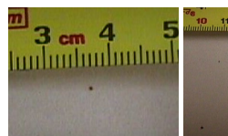
Black Spot 53-gsm newsprint @ 5000 feet/min (1524 m/min)
