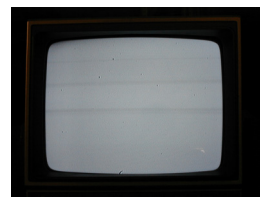
Coating Streak (magnetic media)
