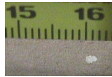
Light Spot 33-lb linerboard @ 2500 feet/min (762 m/min)
