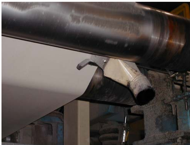
Figure 9 – Proper Installation relative to angle
